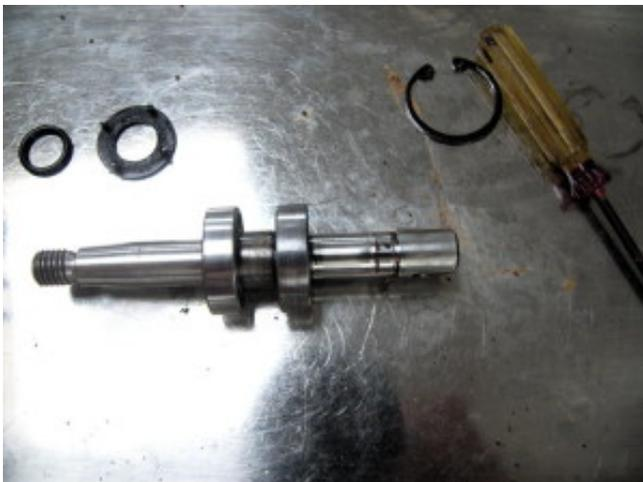
**Step 6 (optional). Modify the new seals.** This picture shows a new seal next to an old one. These lip seals contain a garter spring in them that helps to hold the lip in compression on the shaft. The problem with these springs in this application is that they corrode and lose their functionality. The next picture shows the corroded remains of the spring from our old water seal, along with the sprung
