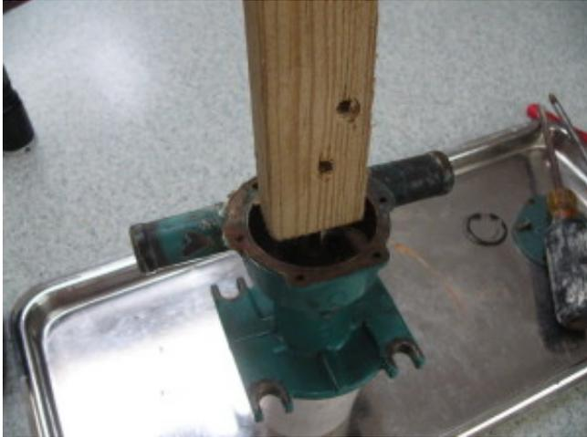
Here is the shaft, bearing assemblies and seals. **PLEASE NOTE:** I removed the seals before taking a picture, so quickly placed them back for a picture. However, I placed the spacer in the wrong direction. So don't use this picture as a guide.
