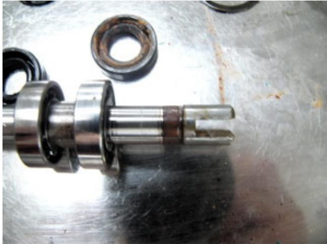
You may have grooves in the shaft where the seal lips wear on it. If these are too deep, you will need to replace the shaft or sleeve it with a speedy-sleeve. In this picture of the (mostly) cleaned shaft, you can see some slight grooves in our shaft. These are not a problem so the shaft was reused.
