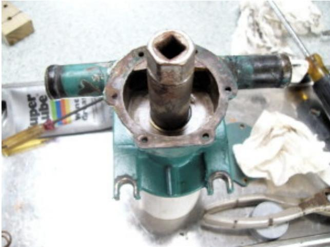
Next, place the spacer on the shaft **with the legs down toward the oil seal and the flat part up toward the water seal.** Place the o-ring on top of the spacer.
