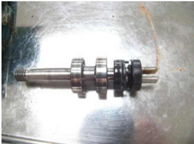
Instead, remember this: the correct orientation for reassembly is oil seal with open end facing aft, followed by spacer with the feet facing aft resting on the oil seal, followed by the o-ring sling washer, followed by the water seal with the open end facing forward.
