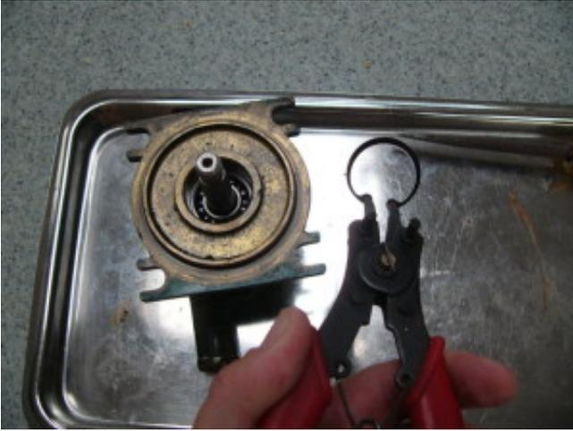
**Step 4. Remove the shaft from the pump housing.** This part is a bit tricky, but not difficult. The problem is that the shaft must be driven back out of the housing while the pump body is supported and the shaft is free. You have many choices of ways to accomplish this. Here, I used a short piece of 2" PVC pipe to support the pump body and allow the shaft to drop free. You can also drill a hole in a piece of wood to allow the shaft to drop through while the wood supports the pump body.
