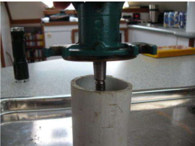
Once the pump body is supported and the shaft is free to drop, place a block of wood on the front end of the shaft and use a mallet to gently tap the shaft out of the pump body. Remember, the shaft is removed through the back of the pump. Don't wang on it! It should tap out fairly easily. If it doesn't because the bearing are corroded to the housing, apply penetrating oil, let sit and try again. If you wallop it, you
