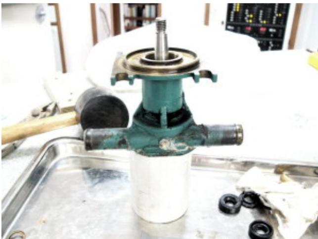
**Step 8. Install the new seals.** The new seals need to be carefully and straightly pressed into the pump body. Put some grease on the shaft to help prevent damaging the seal lips and slide the oil seal onto the shaft **with the open end**
