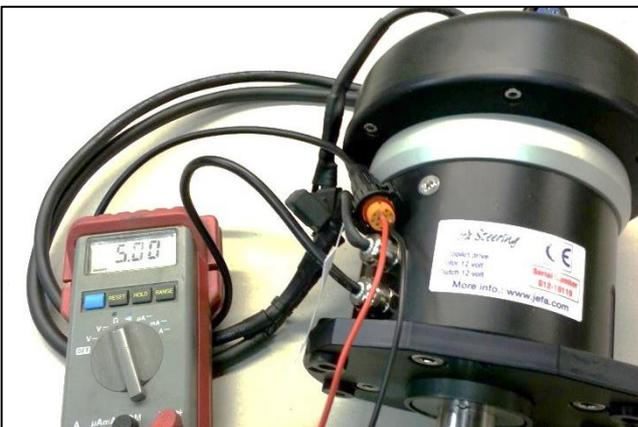
Now turn the steering system from hard over to hard over slowly and check that the multimeter follows correctly.
