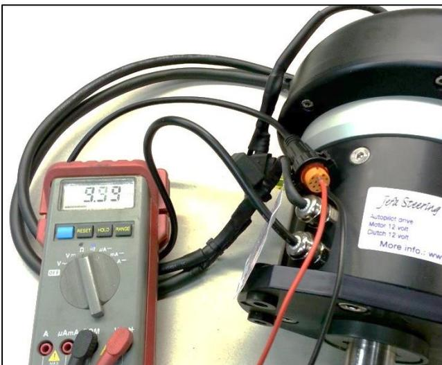
Turn the steering system all the way to opposite hard over to get the highest reading on the multimeter. The multimeter should read from  $8,5k\Omega$  to  $10k\Omega$
