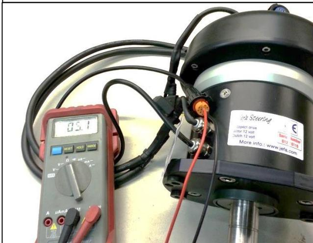
Turn the steering system all the way to hard over to get the lowest reading on the multimeter. The multimeter should read from  $0\Omega$  to  $1,5k\Omega$
