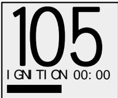
Turn on the ignition, but do not start the engine; the display changes to show that the ignition has been turned on. If left in this state for 30 seconds, the display will flash between WARNING / NO TACH and the alarm will sound in sync with the flashing. The 30 delay only applies when the ignition is first turned on, at any other time a missing tachometer signal (possibly a broken fan belt) will alarm immediately.
