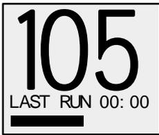
Power on the fuel gauge. After booting up, and assuming the ignition is off and there is fuel in the tank, the display will appear similar to that on the left. The large numbers show the fuel level in litres. The fuel level is also represented by the bar-graph at the bottom. Here this is about 50% of the display width, so indicates that the tank is 50% full. It can be deduced that the tank in this example holds 210 litres.
