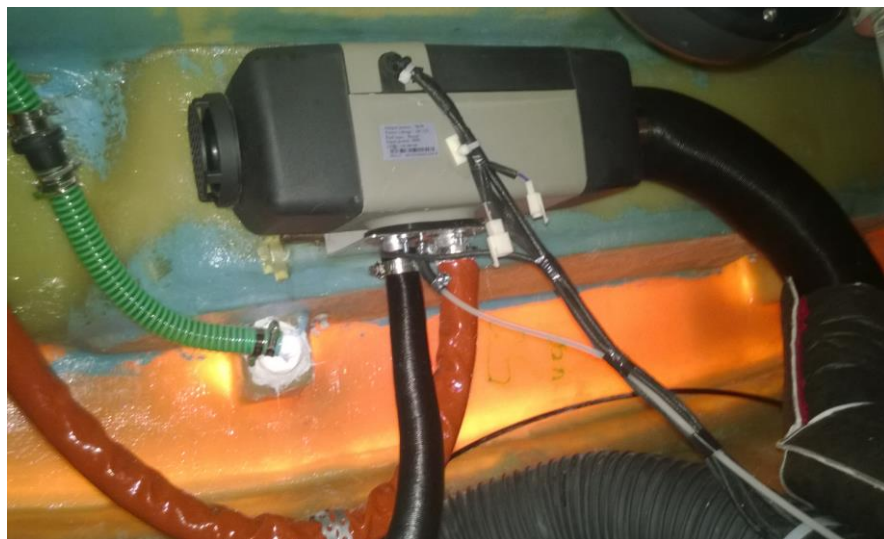
Figure 11 Heater fitted in the aft of the boat
