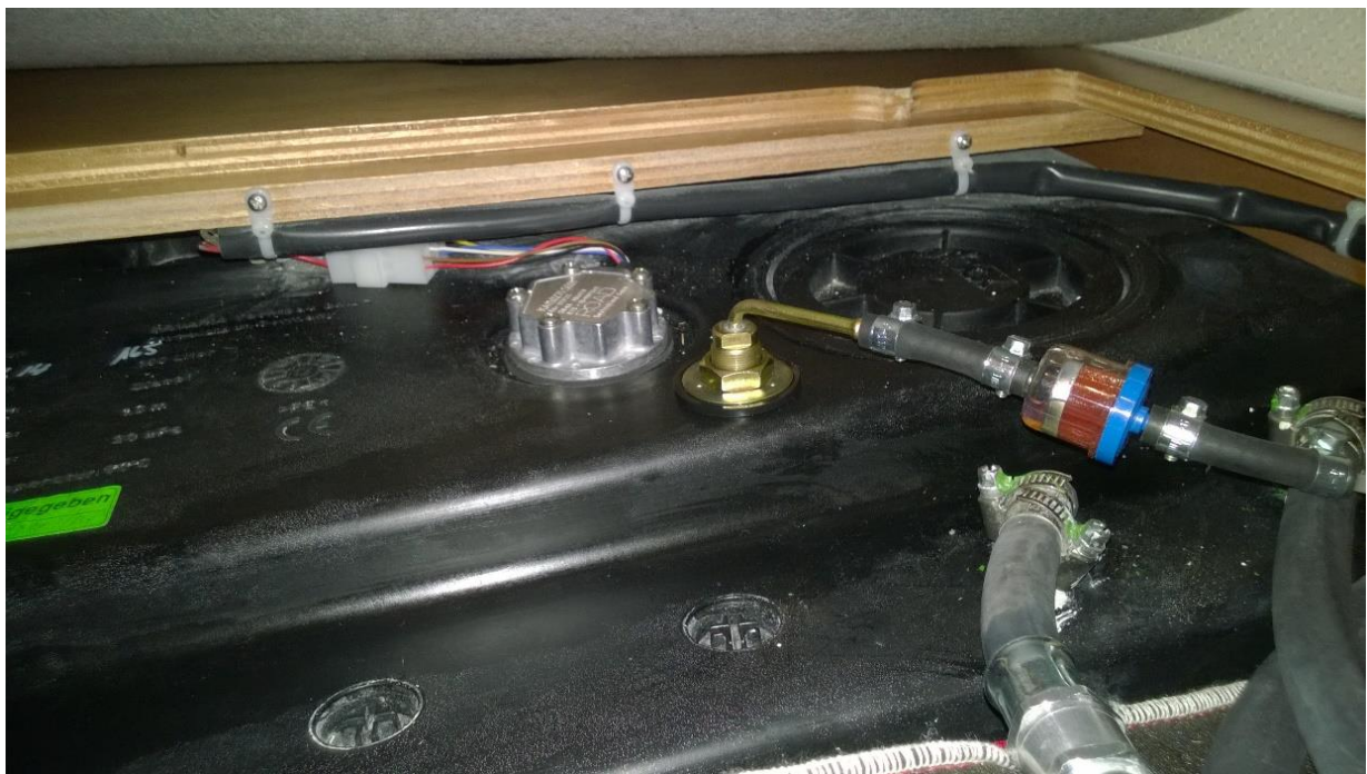
Figure 4 Tank, Supply tube, filter and pipes
