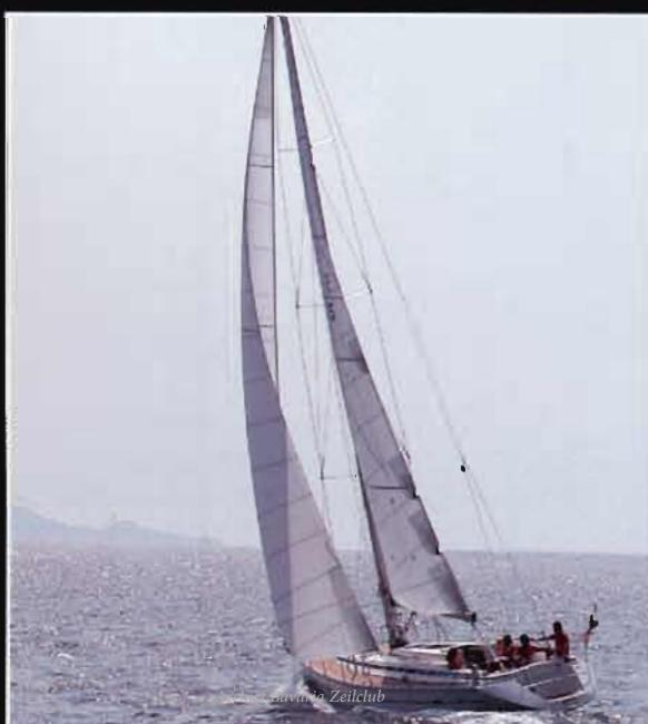
Perfection of drive: Selden rig with battcar system and three spreaders. Touring rig with furling mainsail as an alternative. Can be operated single-handed from the cockpit. Aesthetic and functional: Transom and forebody.
