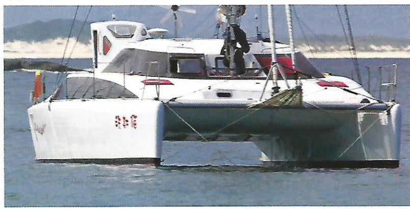
ABOVE: The snubbers on Josepheline are attached to the transom, run through the stanchion bases to a turning block on the bow and then to a common chain hook. This length of snubber gives more than adequate elasticity to absorb the energy of snatch loads.
