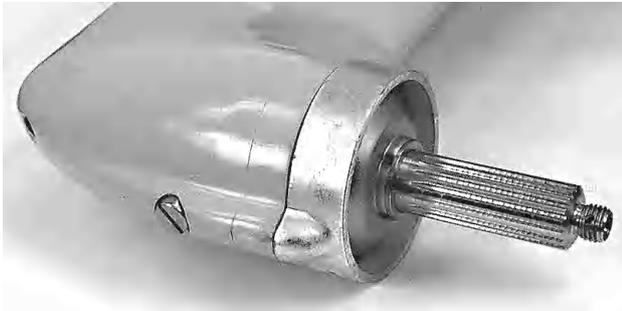
**1.** Clean the outside of the drive. Remove the propeller and remove the fishing line cutter. Unscrew the drain plug and drain off the oil.
