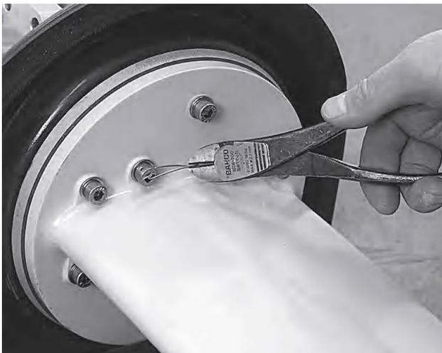
**2.** Remove the locking wire from the four socket cap screws below the division line of the drive, two on each side. Throw the wire away. Then remove all the (10) screws.
