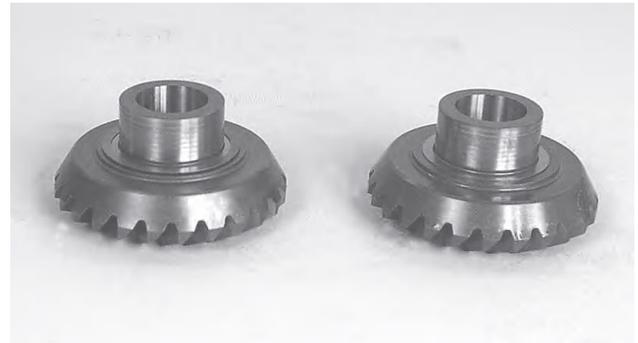
**48.** Put shims on the gear wheels for the upper bearing housing and gear housing. Start off with 0.50 mm for each gear wheel. This is a value which is based on experience.
