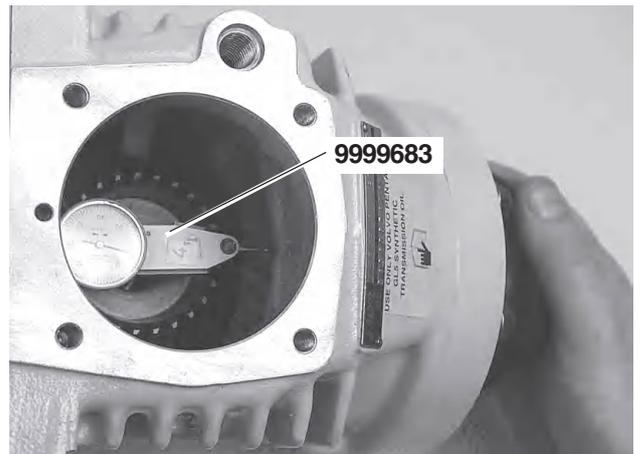
**87.** Measure the flank clearance with a dial gauge and rocker **9999683**.
