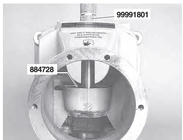
**95.** When the correct pre-load has been obtained, remove the lower bearing cover, the slipping clutch and the small outer bearing in the gear housing.
