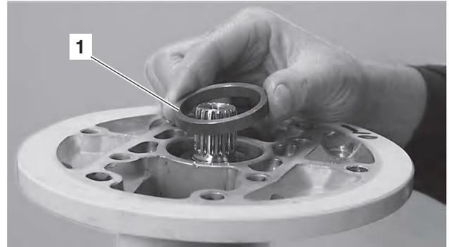
**3.** Separate the upper and lower gear housings. Remove and scrap the gasket at the division line. Remove the shims. Note the number of shims. Remove the spacer ring (1). Tap the shaft lightly with a plastic-faced hammer.
