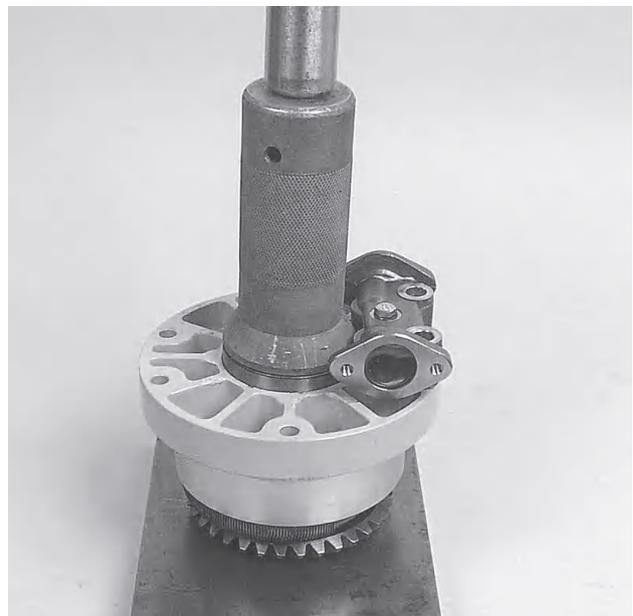
69. Apply sealant, Volvo Penta part. no. 840879-1 on the mating face of the seal ring against the bearing housing.
