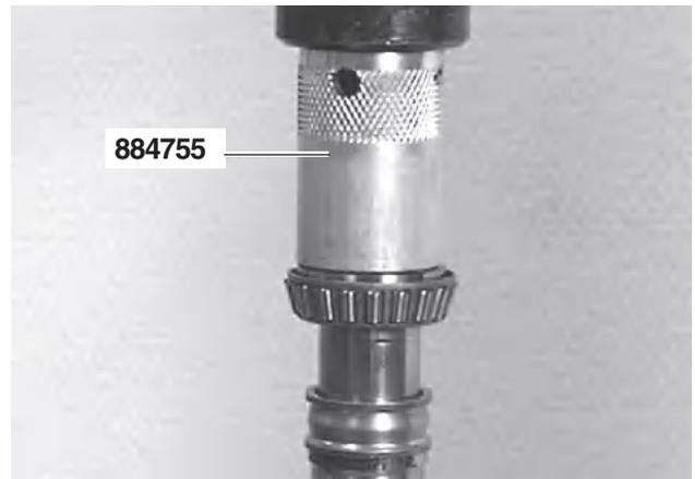
18. Install a new roller bearing with mandrel **884755**.
