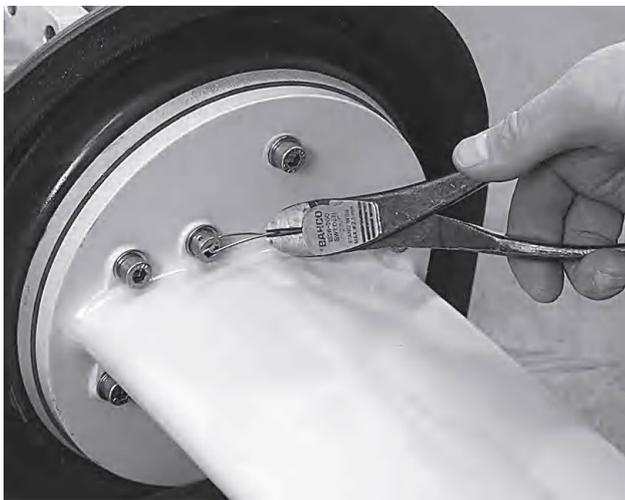
**2.** Remove the locking wire from the four screws. Then remove all the screws, 10 pcs below the division line of the drive.
