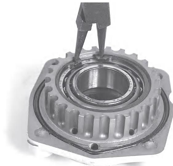
**47.** Install the circlip, using circlip pliers. Turn the chamfered side down, towards the gear housing. Make sure that the circlip is securely seated in the groove.
