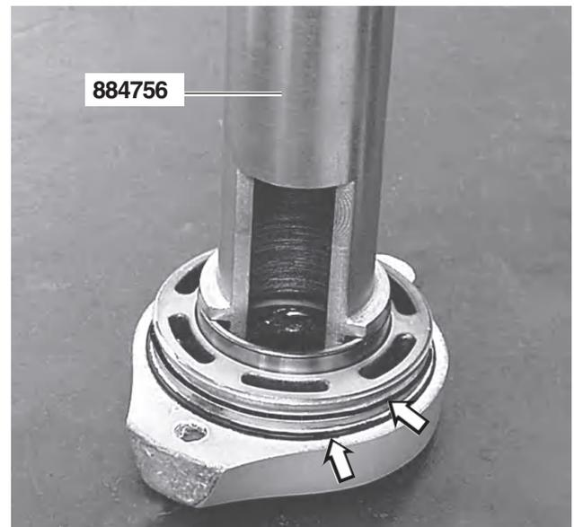
**40.** Assemble the outer bearing race with tool no. **884756**.
