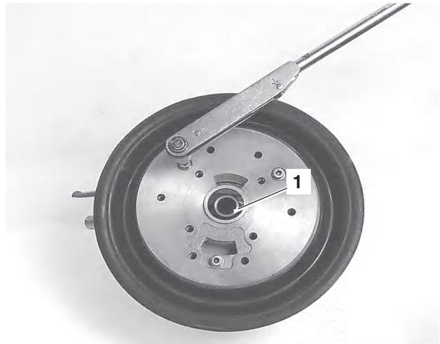
73. Install the adapter plate on the upper gear housing. Apply MoS2 based grease, Volvo Penta part no. 1161029-2 to the three socket cap screws. Put washers on the socket cap screws and use a torque wrench to tighten them. Torque the screws alternately. Tightening torque: **30 Nm (22.13 lbf ft)**. Install the slipping clutch (1).
