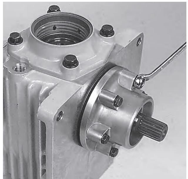
**119.** Put a new O-ring and the tested thickness of shims on the input bearing housing.
