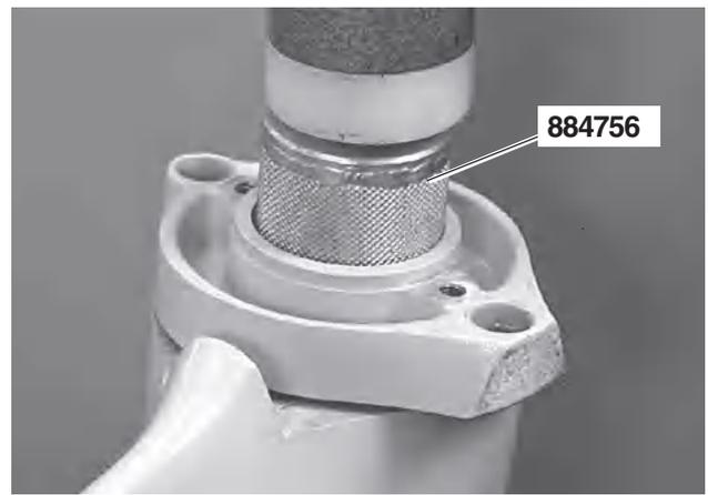
**31.** Install the outer bearing race in the gear housing with mandrel **884756**. Use the rear bearing housing as a guide.
