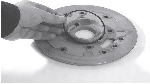
72. Oil and install a new O-ring on the adapter section neck.
