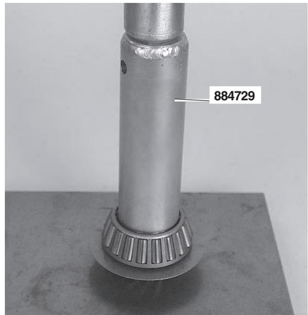
38. Press the large roller bearing onto the drive shaft. Use tool no. **884729**.
