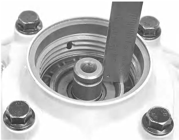
**112.** Measure the distance between the gear wheel and the bearing.
