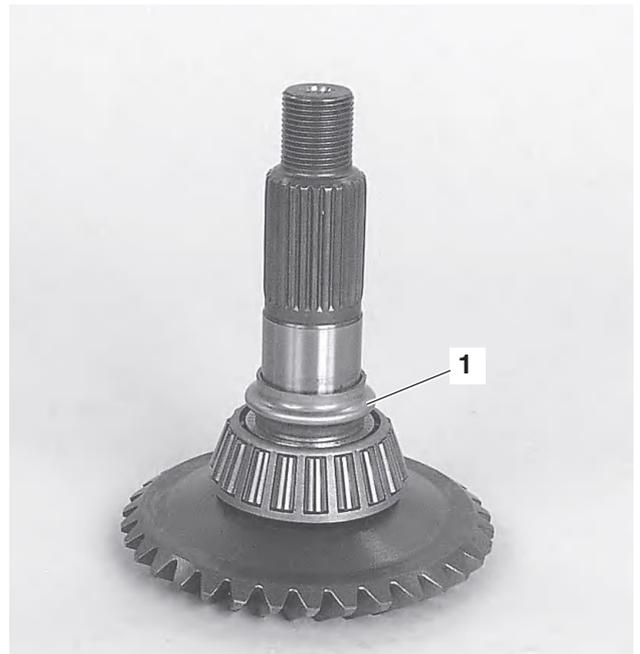
57. Remove the ferrule (1) from the output shaft.
