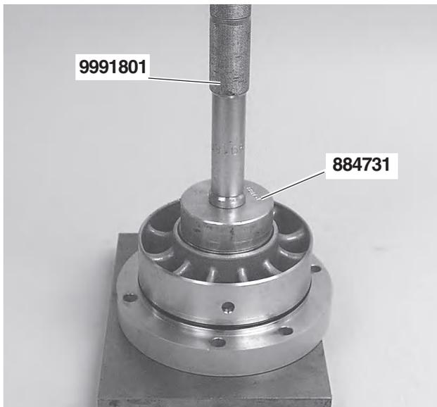
62. Install one of the outer bearing races in the bearing housing. Use tool no. **884731** and shaft **9991801**.
