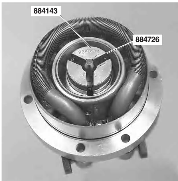
59. Remove the outer bearing races from the output bearing housing. Use tool no. **884726** and shaft **884143**.
