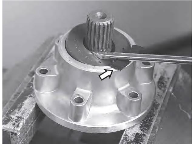
29. Fix the bearing housing in a vise. Press a screwdriver into the seal ring. Then place a thick piece of rubber or leather between the screwdriver and the bearing housing casting. Prize out the seal ring and scrap it.
