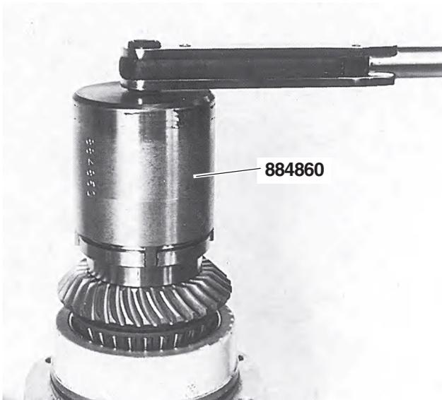
**28.** Screw two screws into the tubular shaft and fix it in a vise. Align the tubular nut with the un-threaded section towards the crown wheel and install it with tool no. **884860**.
