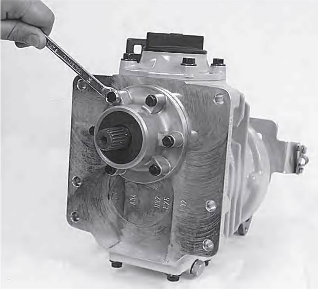
**14.** Disassemble the double bearing seal housing, 6 screws.
