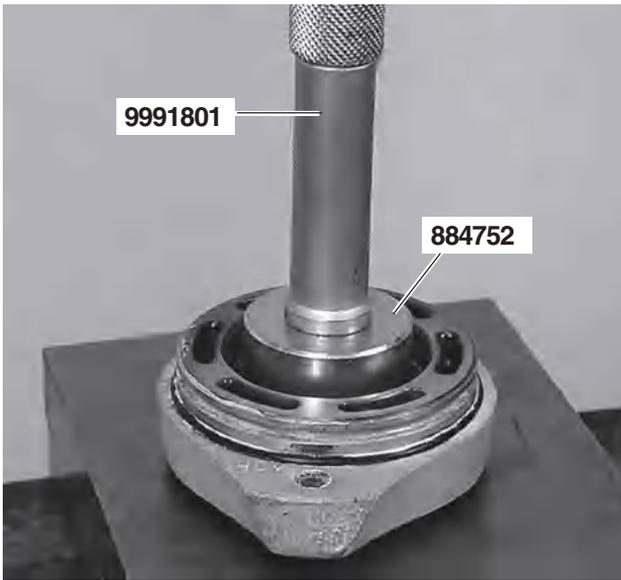
**36.** Install a new seal ring in the bearing housing, using tool no. **884752** and shaft **9991801**. Apply sealant, Volvo Penta part no. 1161099-5, to the mating face between the seal and the bearing housing.
