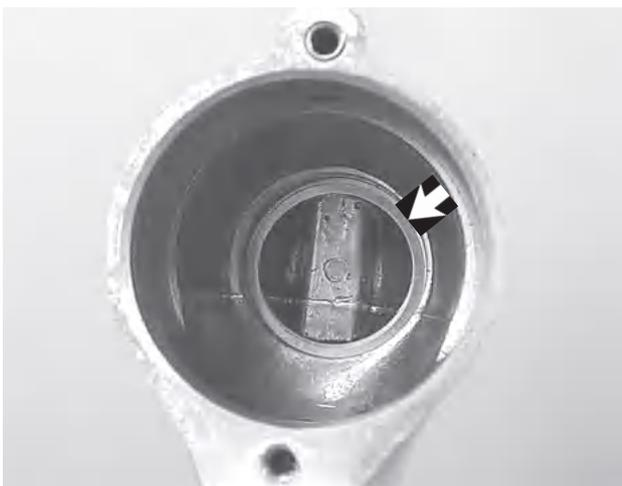
**30.** Put shims of the correct thickness in the lower gear housing. Add a further 0.05 – 0.10 mm. In this case, we put a total of 1.00 mm shims in the housing.
