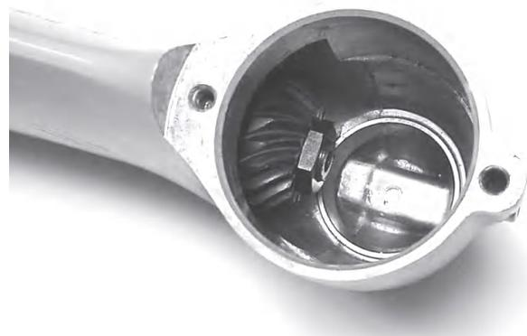
**45.** Install the vertical shaft in the housing. Be careful to ensure that the needle rollers do not fall out. Then install the pinion. Apply thread locking fluid, Volvo Penta part no. 1161075-5, on the threads and install the nut.
