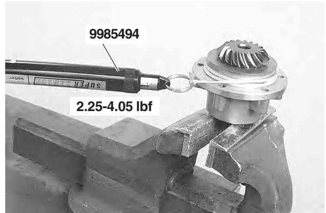
**41.** Test the pre-load with a spring balance. Fix the gear wheel or shaft in a vise with soft jaw pads. Wind a string round the bearing housing, and pull with spring balance no. **9985494**.
