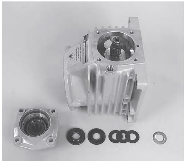
21. Remove the cover. A lock washer, a large spring washer, three small spring washers and possibly one or two spacers will come away with the cover. In addition, the ball bearing and gear wheel are fixed to the cover.
