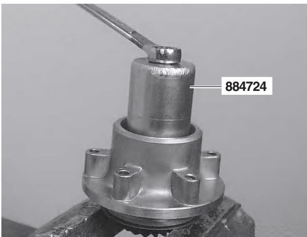
**40.** Screw a new nut on. Turn the chamfer inwards.
