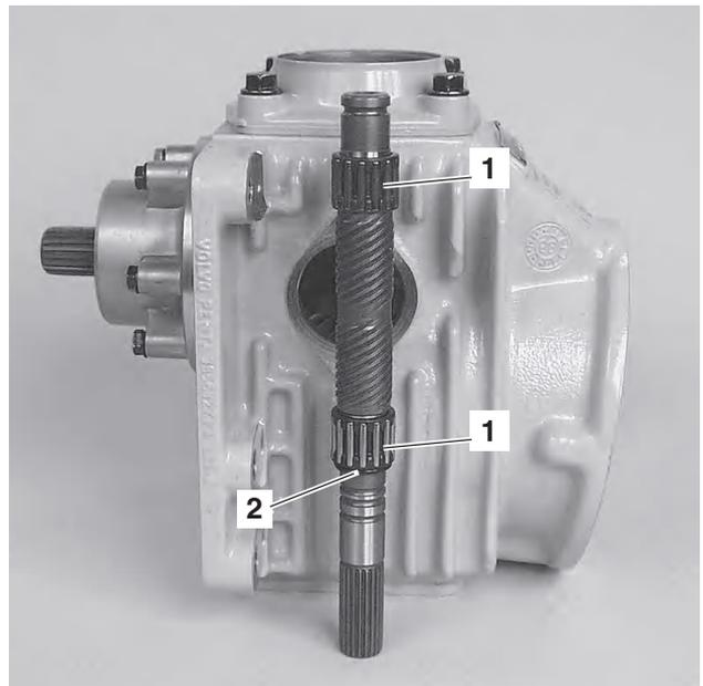
99. Put the vertical shaft, with needle roller bearing, in the housing. The lower needle roller bearing is retained by a rubber band or O-ring.
