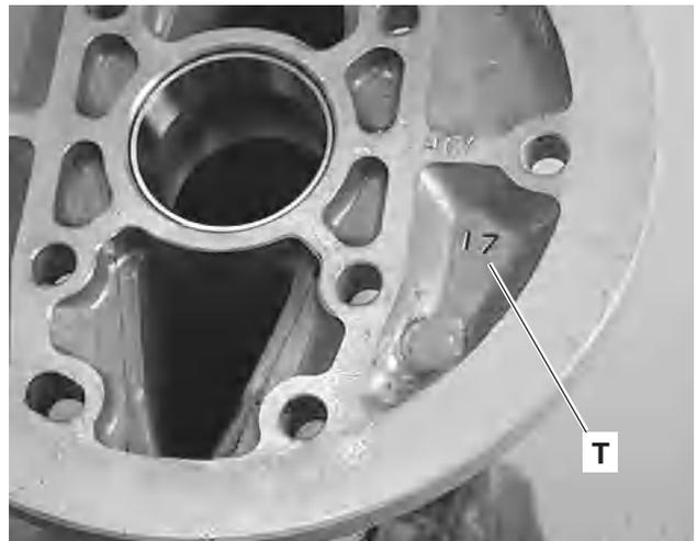
28. Dimension (**T**) is stamped on the starboard side of the gear housing division to permit the shim thickness under the front bearing race to be calculated, which is 17 in this case. The dimension of the division plane can vary between 0 and 30.
