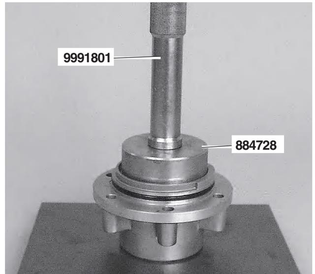
**33.** Drive out the small outer bearing race, using tool **884728** and shaft **9991801**.
