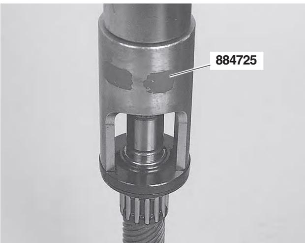
24. Put the vertical shaft in a press and press the large washer with tool no. **884725**, to release the retention ring halves. Remove the halves.
