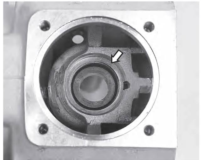
79. Place the shims, as calculated, in the housing. In this case, they are 0.40 mm.
