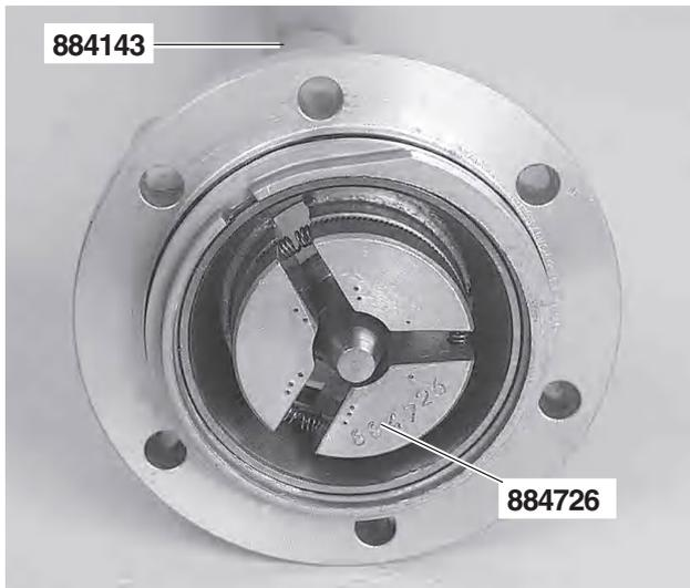
**32.** If the roller bearings are damaged, they must be changed. Remove the large outer bearing race from the bearing housing, using tool no. **884726** and shaft **884143**.
