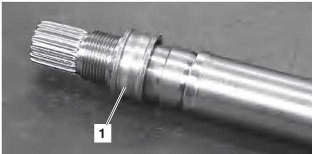
15. Remove the ferrule (1). Use a knife puller as a counterhold.
