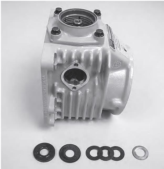
**113.** Put on, from the left, the measured spacer washer, three small domed washers, a large domed washer and the lock washer.
