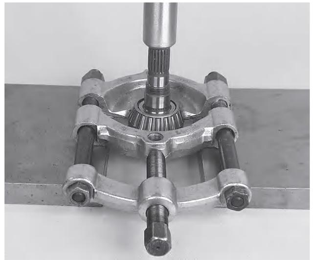
**34.** Remove the roller bearing from the input shaft, using a knife-type extractor. Then remove the washer. Clean the components and check for wear, replace worn and damaged components.
