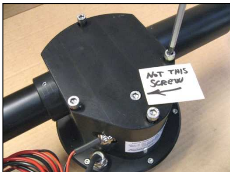
Unscrew 4pcs of screw. NB!! Do not dismount screw in the center, only 4pcs in edge
