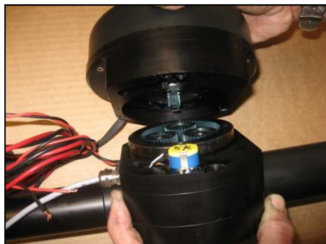
Assemble housings, and make sure that the gearwheels are fitting
