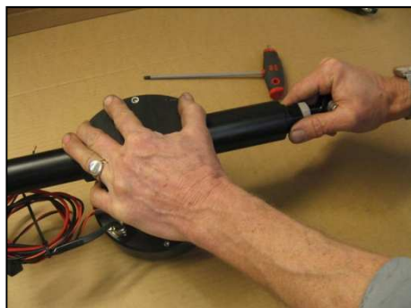
Push drive arm in to stop. Installation of the rudder feed back is done.
