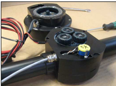
Assemble the cable screw to hold the cable for rudder feed back
