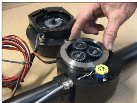
Take gearwheel from top housing and mount it on the gearwheels on bottom housing
