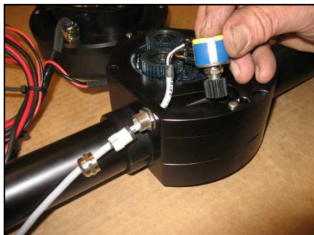
Mount the rudder feed back. NB!!! Do not use hammer on rudder feed back, only use hands
