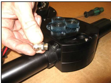
Pull out plastic plug to mount the cable screw
