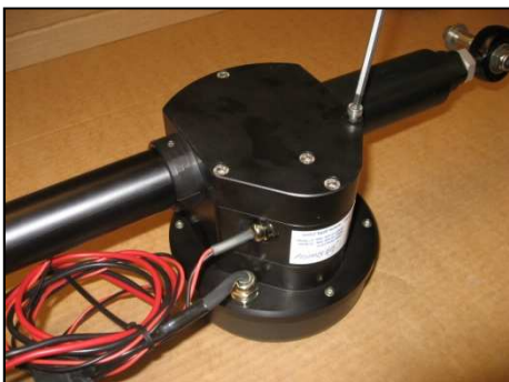
Mount 4pcs of screw to assemble the drive unit
