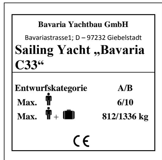
The boat Bavaria Cruiser 33 "has been tested according to ISO 12217-2 regarding stability and freeboard, buoyancy and swimming ability. Hence the various stipulations about the number of people and the payload. The builder's plate which is mounted on the dashboard next to the steering position, looks as follows:
