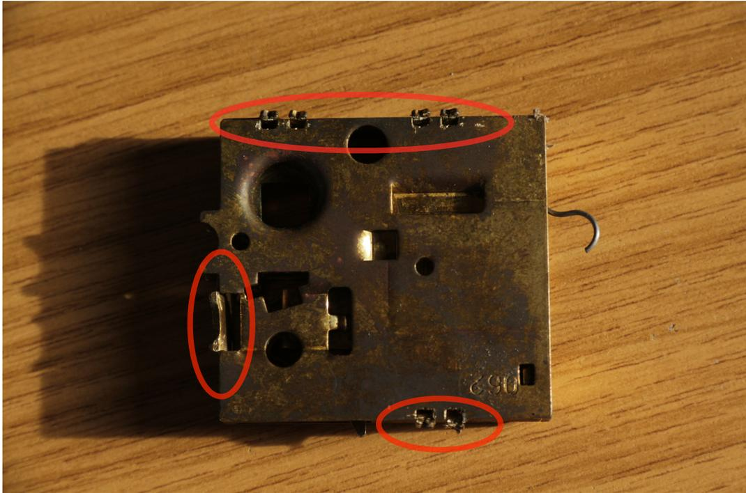
Cabin latch with the face plate and striker removed. Tabs holding top plate to lower body have been bent back so that top plate can be removed.
