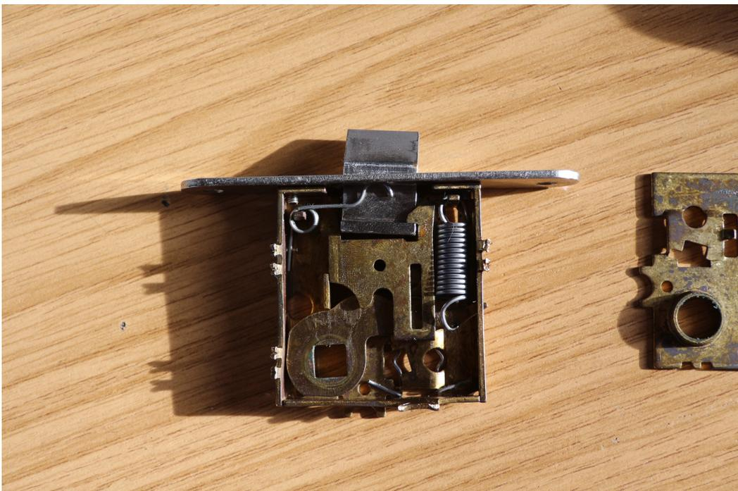
re-assemble. Then fit the striker plate ensuring it is the correct way round then attach the face plate. Top cover was then fitted and the small tabs tapped back into position to hold it all together.
