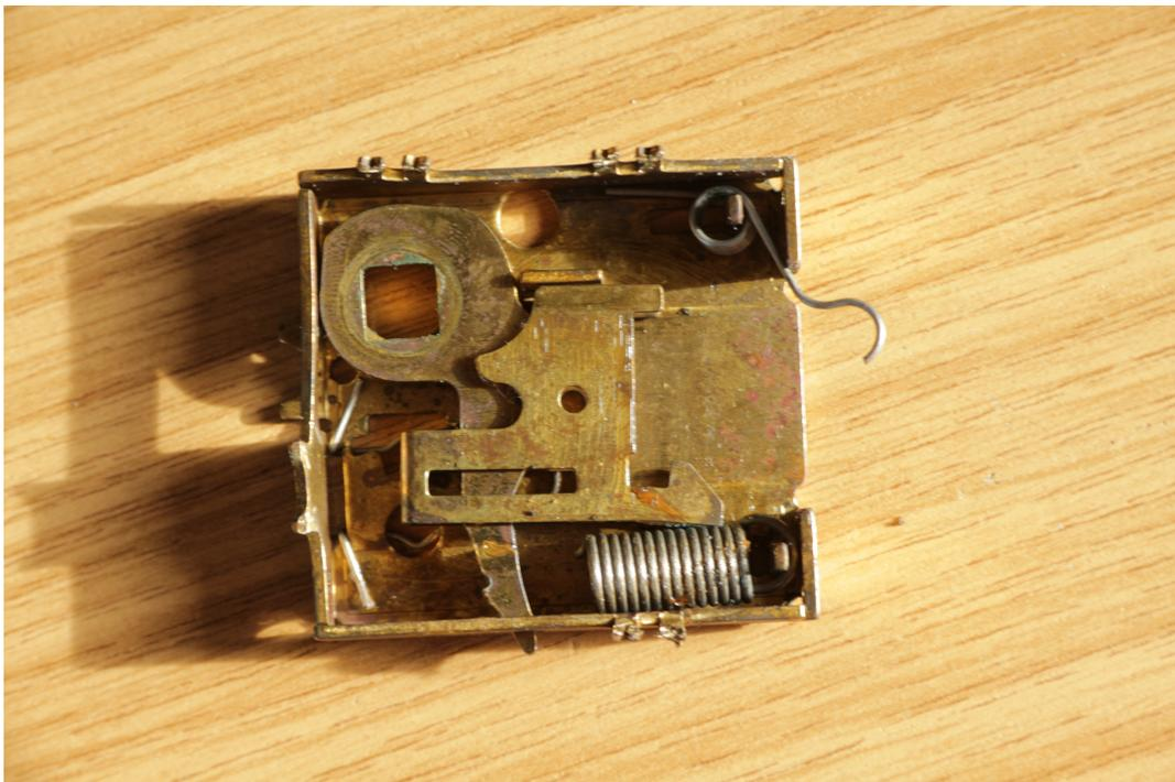
Top plate now removed broken spring can be seen bottom left.
