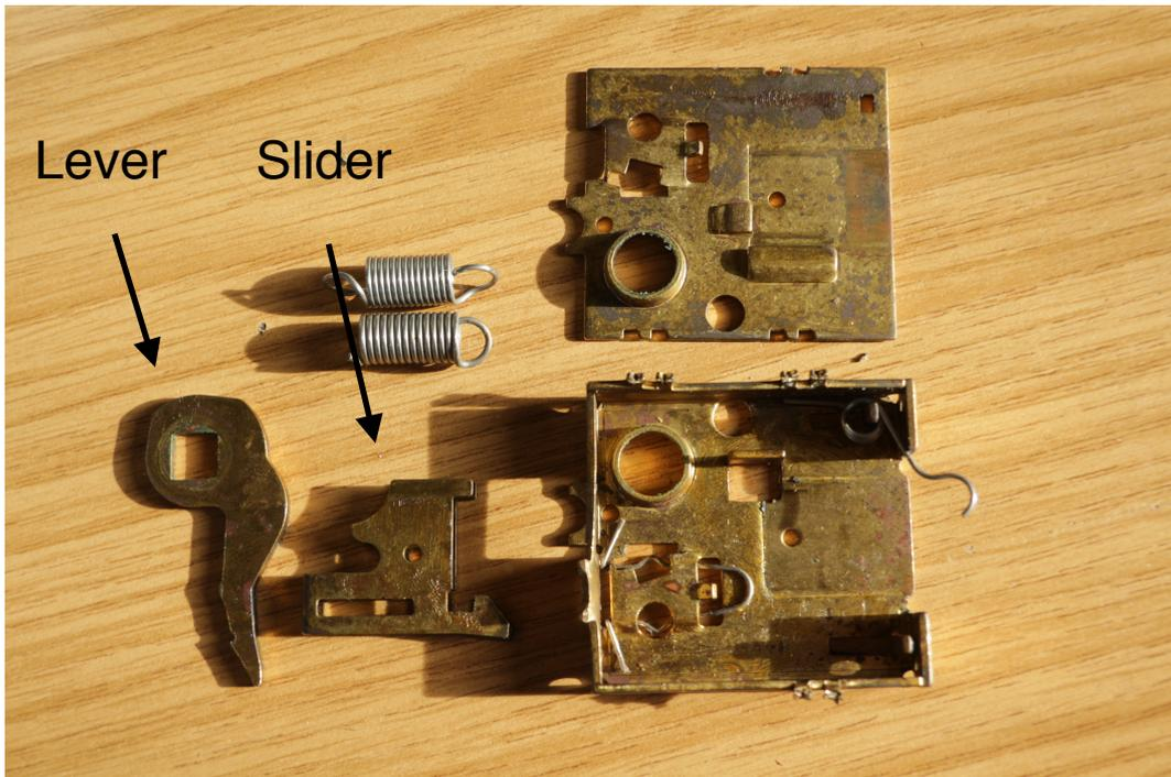
Component parts now removed, broken spring shown alongside new.
