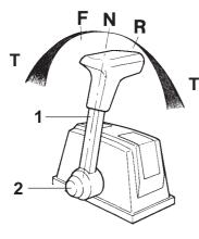
Control lever for tip mounting
