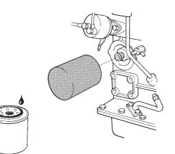
Unscrew the old filter. (To avoid oil spills put a plastic bag over the filter before it is unscrewed). Check that the engine mating surface is clean. Moisten the filter rubber gasket with a little oil. Screw on the new filter by hand until it is in contact with the mating surface. And then a further half turn but no more!
