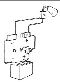
5. If an auxiliary battery is in use, a main switch (D) should be connected between its + terminal and the fuse block. The main switch for the auxiliary battery must cut off all power consuming equipment connected to that battery and be turned off when power is no longer needed.
